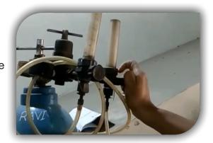
When the flow on the front of the analyzer is showing "ZERO" reading, then disconnect the tubing from the cylinder
