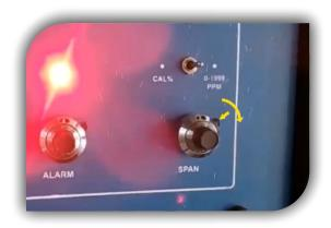
Turn off gas flow from the cylinder by closing the needle valve
