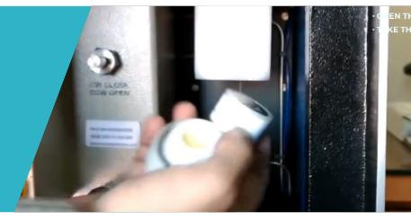
Put back the cleaned filter back in housing
