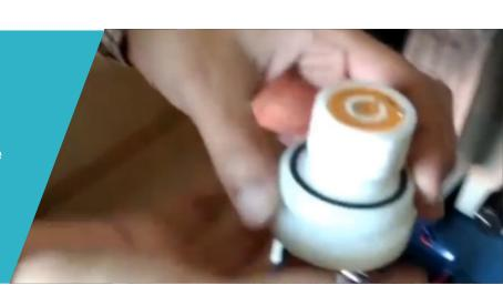
Tighten sensor holder nut
