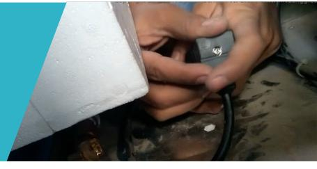
• Fit the auto-drain back with allen key and screw
