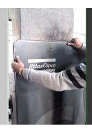
Remove the Side Cover of Air Compressor
